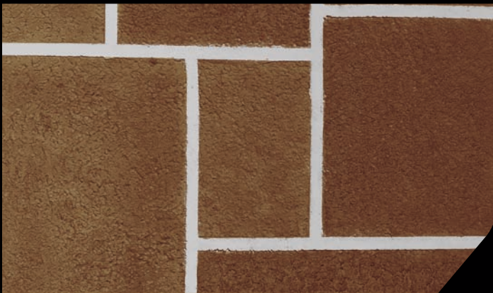
BASE: 2/3 DT25 in 2 lt FONDO UNIVERSALE - 1 DTX08 in 4 lt OLD FASHION - FINISH: 1 DTX08 in 750 ml VELE' + SHADE' L BRONZO
