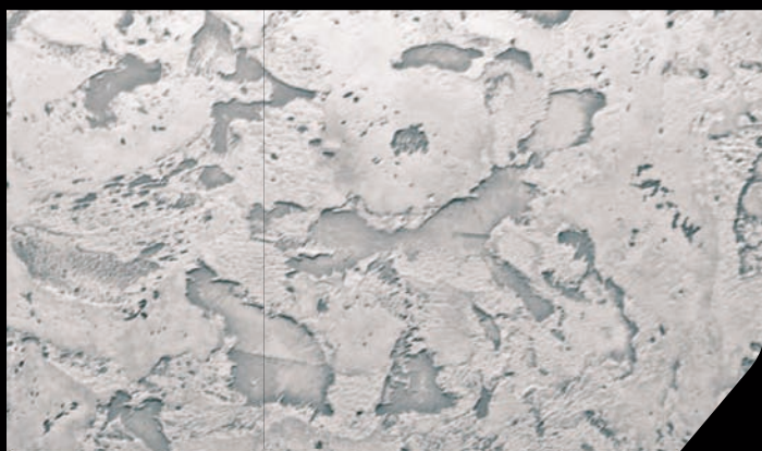
BASE: 1 DT96 in 4 lt OLD FASHION FINISH: 1/3 DT04 in 750 ml SHADE' L ARGENTO
