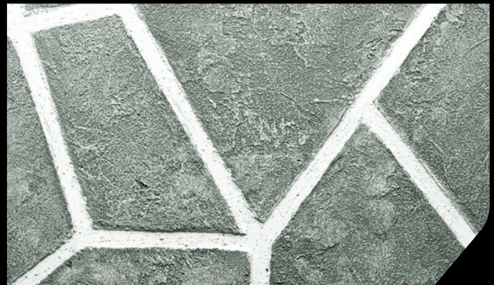
BASE: 2/3 DT25 in 2 lt FONDO UNIVERSALE - 1 DT25 in 4 lt OLD FASHION FINISH: 1 DT93 in 750 ml VELE' + 1 DT25 in 750 ml VELE'
